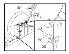
the Magnet (58) on the flywheel. Retighten the Screw. Turn the left Pedal Disc (15) for a moment. Repeat until the console displays correct feedback.
