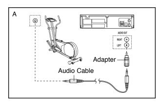
B. Plug one end of the audio cable into the jack beneath the console. Plug the other end of the audio cable into the adapter. Plug the adapter into an RCA Y-adaptor (available at electronics stores). Next, remove the wire that is currently plugged into the AUDIO OUT jack on your VCR and plug the wire into the unused side of the Y-adaptor. Plug the Y-adaptor into the AUDIO OUT jack on your VCR.
