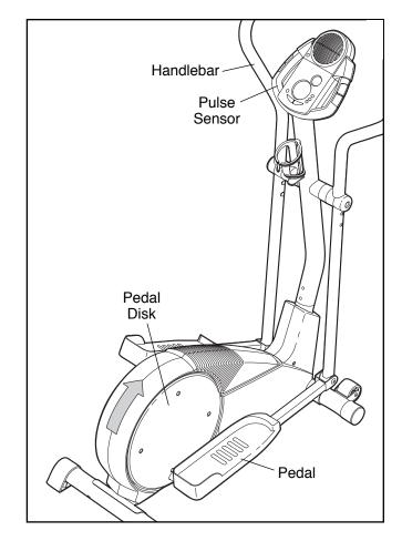
To dismount the elliptical trainer, allow the pedals to come to a complete stop. Note: The elliptical trainer does not have a free wheel; the pedals will continue to move until the flywheel stops. When the pedals are stationary, step off the highest pedal first. Then, step off the lowest pedal.
