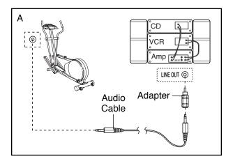
B. Plug one end of the audio cable into the jack beneath the console. Plug the other end of the audio cable into the adapter. Plug the adapter into an RCA Y-adapter (available at electronics stores). Next, remove the wire that is currently plugged into the LINE OUT jack on your stereo and plug the wire into the unused side of the Y-adapter. Plug the Y-adapter into the LINE OUT jack on your stereo.
