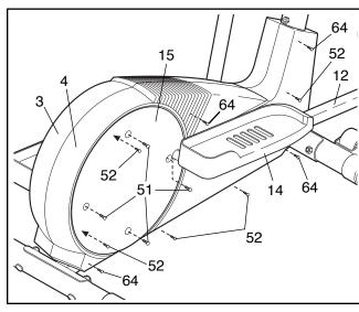
Next, remove the four Screws (51) from the right Pedal Disc (15), and slide the Pedal Disc off. Remove all Screws (52, 64) from the Right Side Shield (4), and remove the Right Side Shield. Remove all Screws (52) from the Left Side Shield (3) and remove the Left Side Shield.
